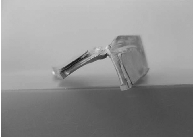
FIGURE 7 Specimen 133 after impact test (front view of fracture surface).
