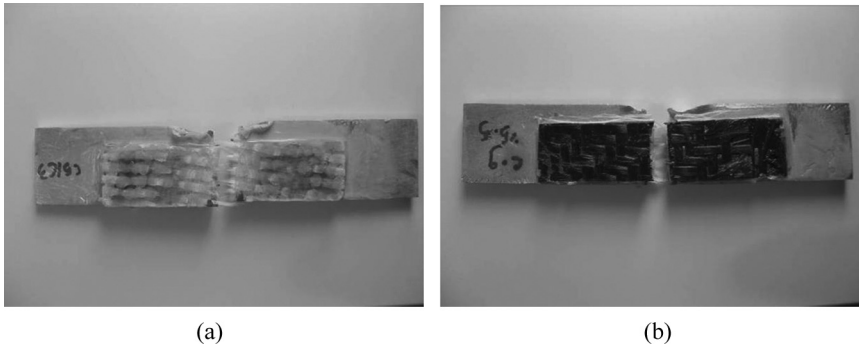
FIGURE 12 Specimen 5215 after impact test (a) Top view, (b) Back view.
